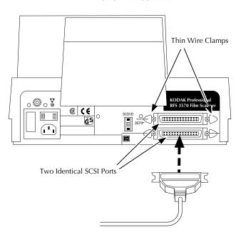
4. Attach a SCSI terminator (supplied with the Scanner) to the empty SCSI port on the Scanner, seat the terminator firmly, and then pinch the thin wire clamps shut.
